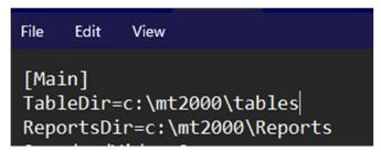
So based upon the above example the tables are in c:\mt2000\tables and the NET DIR in the Borland Database Engine (BDEADMIN) would be "c:\mt2000."
